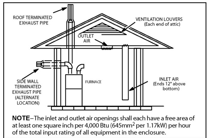
**Figure 7. Equipment in Confined Space - All Air from Outside**
