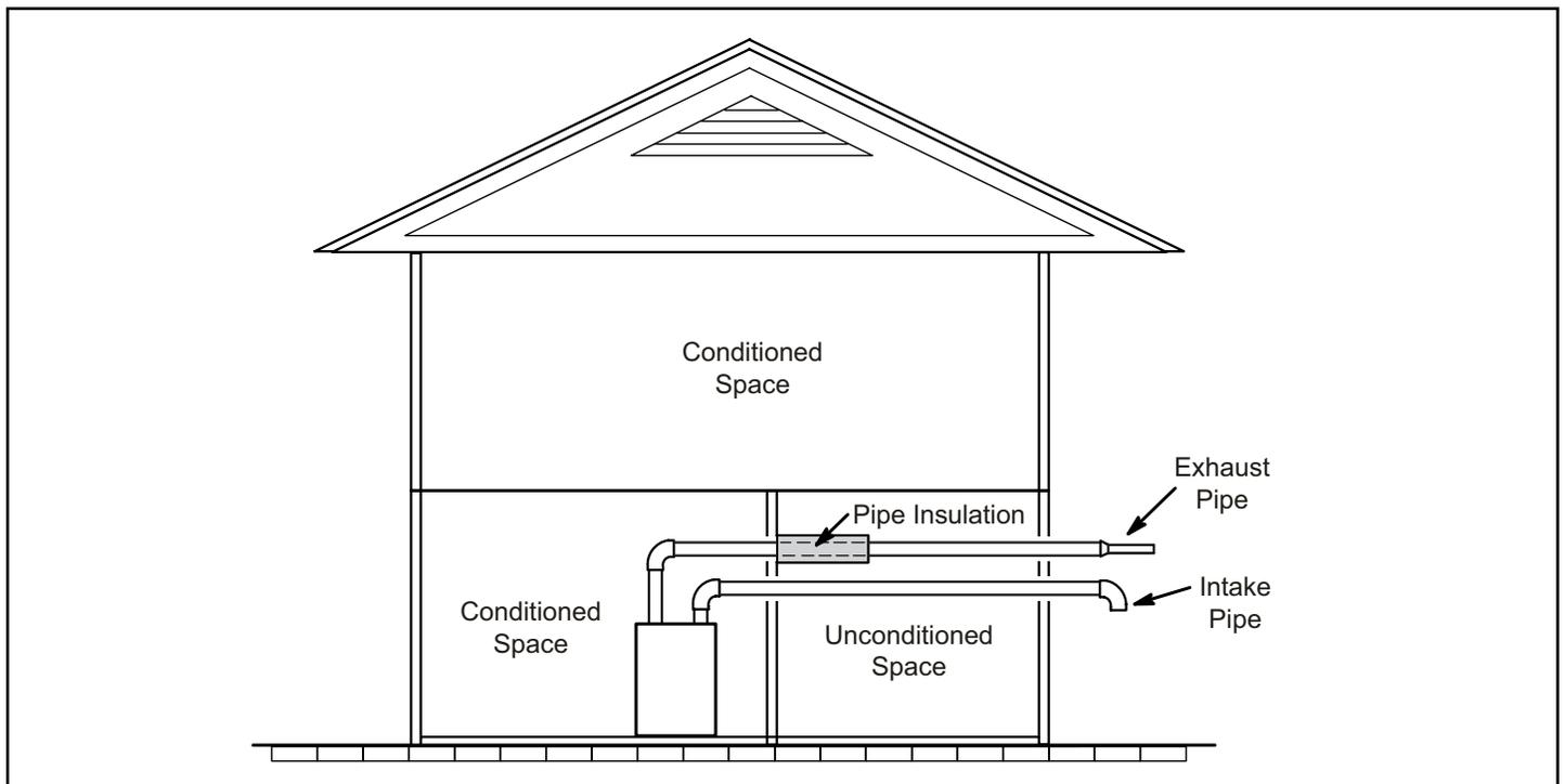
**Figure 33. Insulating Exhaust Pipe in an Unconditioned Space**
