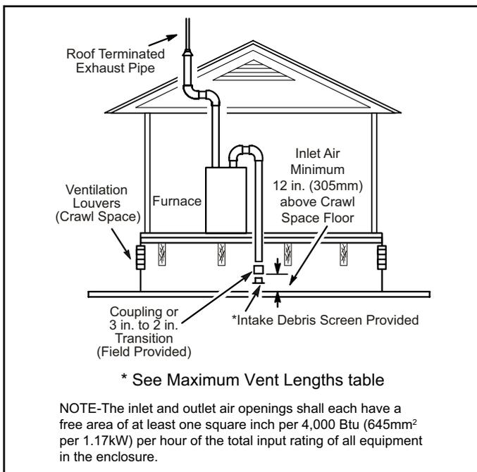
**Figure 10. Equipment in Confined Space
