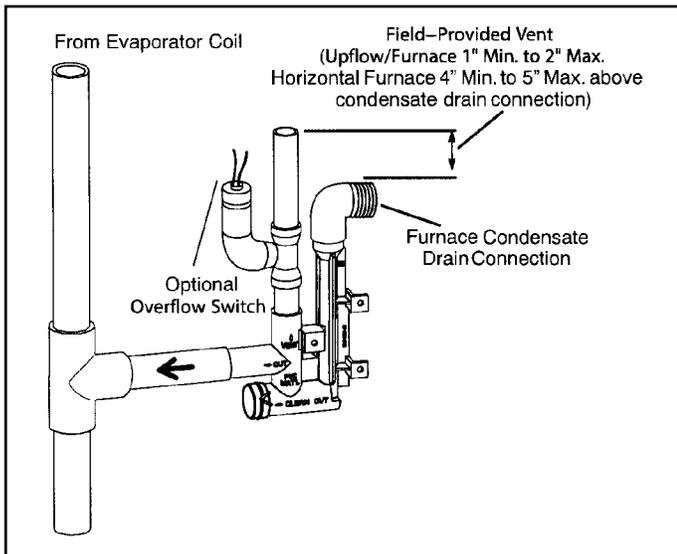
**Figure 54. Condensate Trap with Optional Overflow
