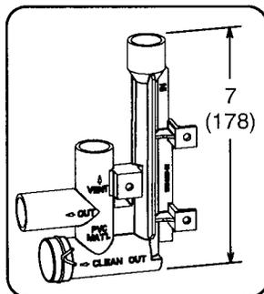
Drain Trap Assembly with 1/2 inch Piping
