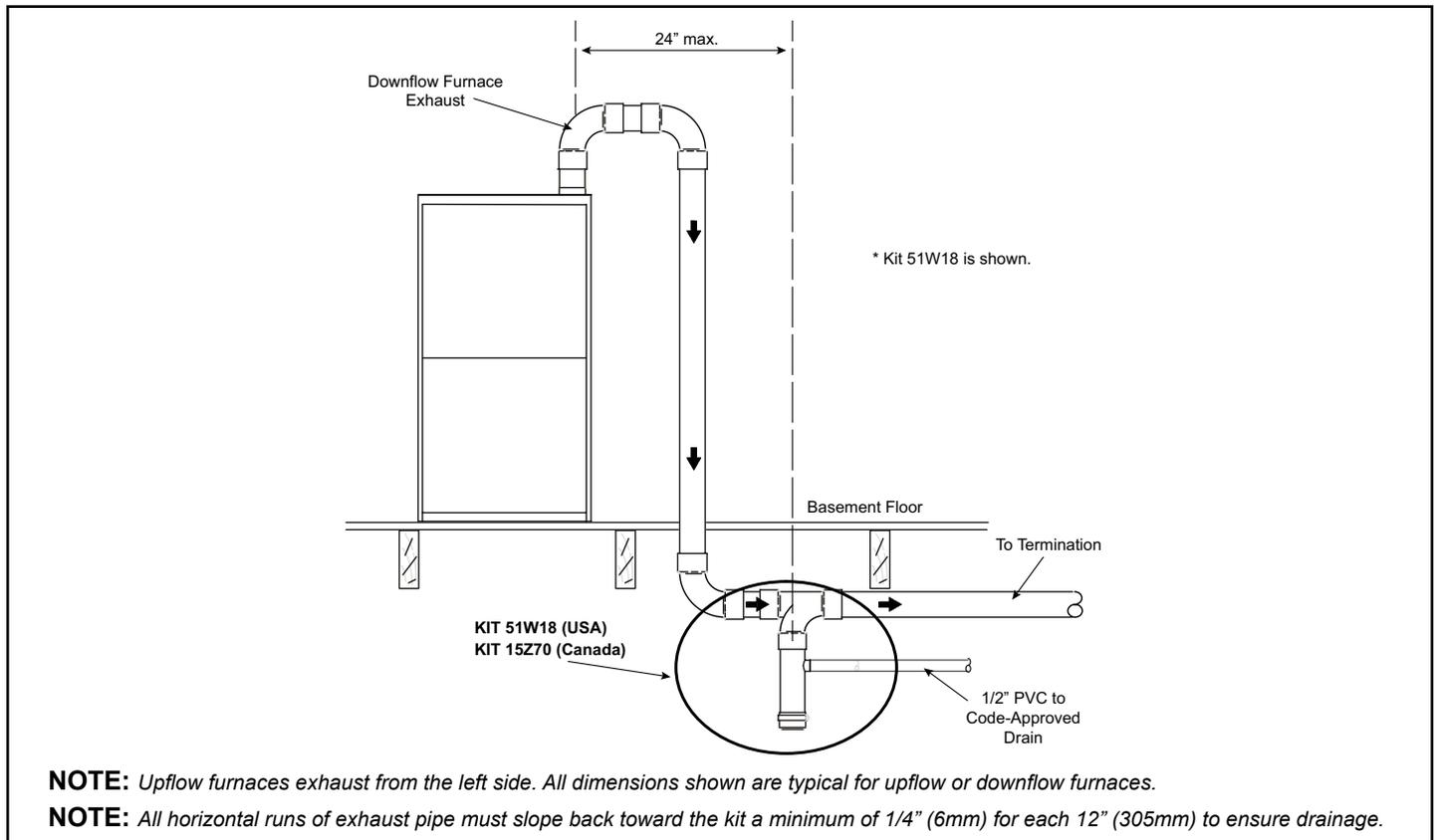
**NOTE:** Upflow furnaces exhaust from the left side. All dimensions shown are typical for upflow or downflow furnaces.
