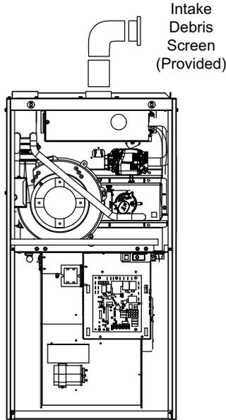
**NOTE:** Debris screen and elbow may be rotated so that the screen may be positioned to face forward or to either side.
