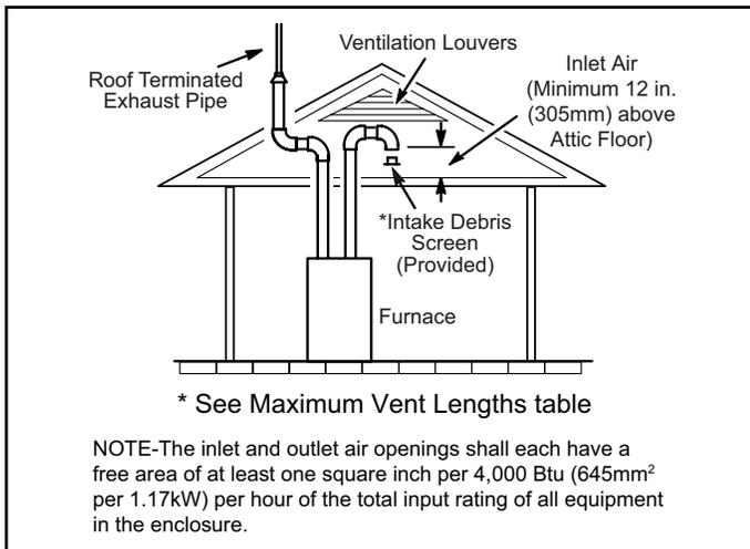
**Figure 9. Equipment in Confined Space
