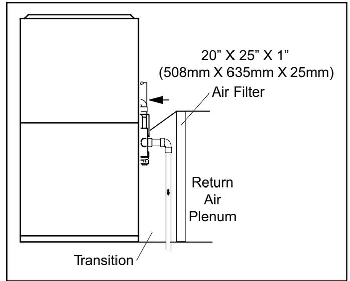
**Figure 14. Side Return Air (with Transition and Filter)**
