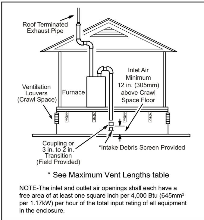
**Figure 32. Equipment in Confined Space
