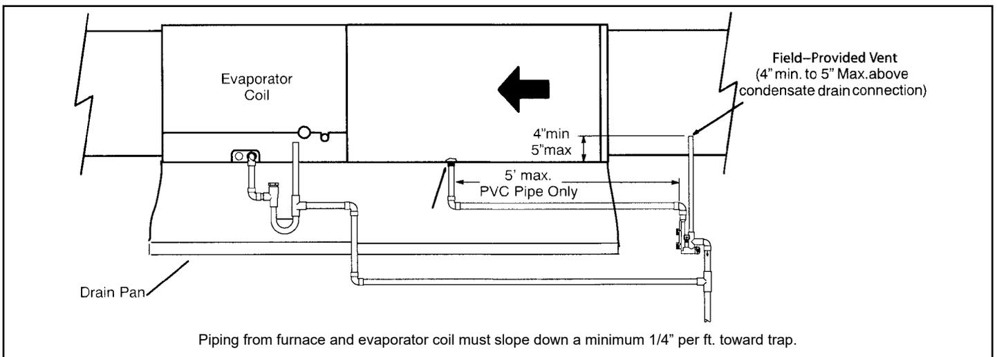
**Figure 58. Evaporator Coil Using a Common Drain**
