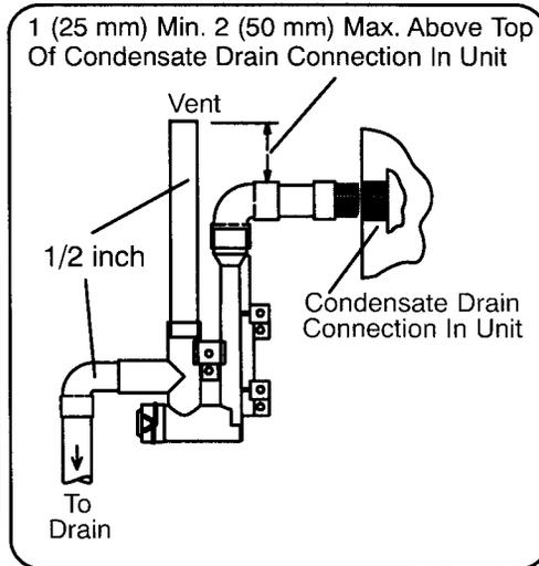
Drain Trap Assembly with 3/4 inch Piping
