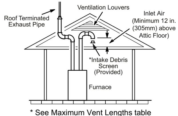
**NOTE-**The inlet and outlet air openings shall each have a free area of at least one square inch per 4,000 Btu (645mm<sup>2</sup> per 1.17kW) per hour of the total input rating of all equipment in the enclosure.
