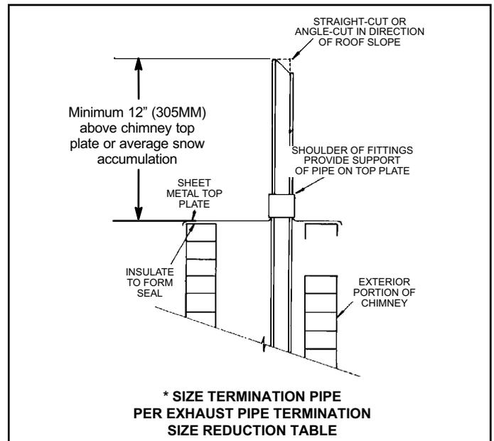
**Figure 48. Non-Direct Vent Application Using Existing Chimney**
